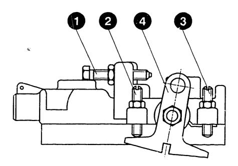
ADJUSTING LOW-IDLE SPEED REGULATION \* Pump with LFG
